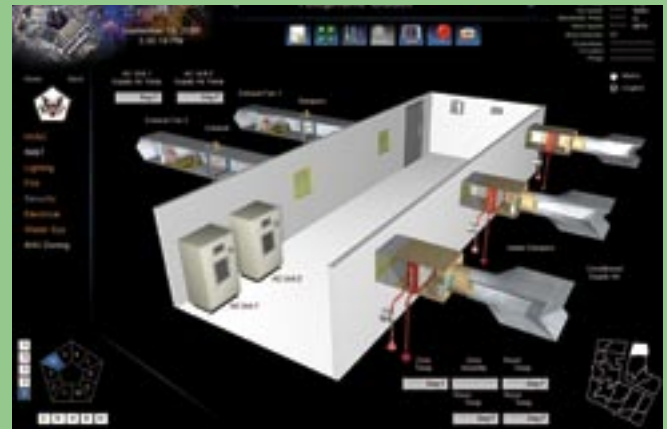
A Building Operations Control Screen
