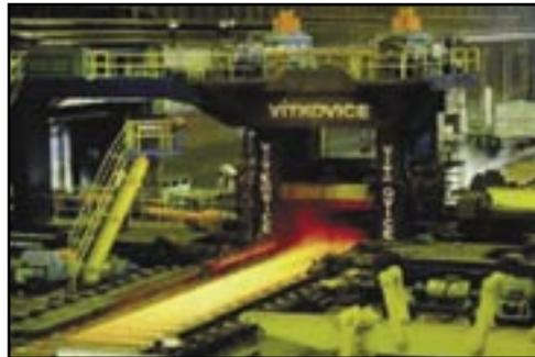
3.5 Meter Four-High Rolling Mill
