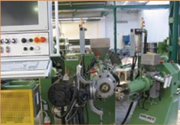
A Cable Line Extruder
