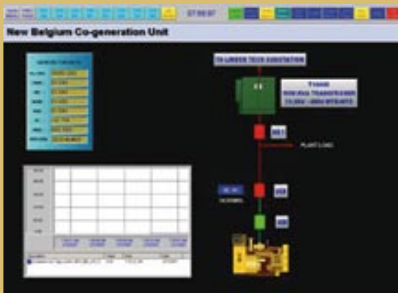
Co-Generation Monitoring at Fort Collins Utilities
