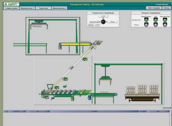
Brick Transport Controls
