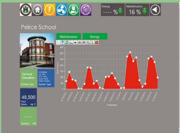
The Peirce School's Main Control Screen, Generated Via GENESIS64™
