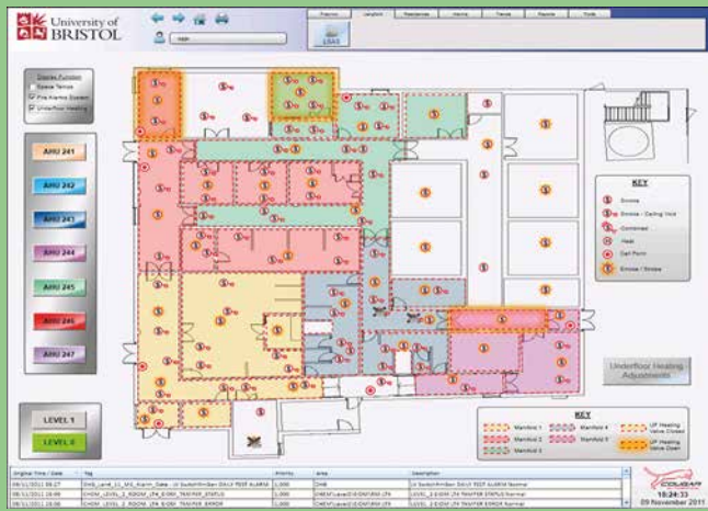
An AHU Zone Monitoring Display
