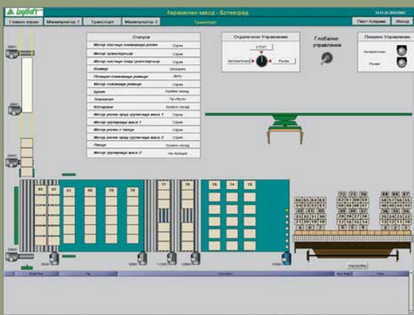
A Factory Control Screen at The Ceramic Factory
