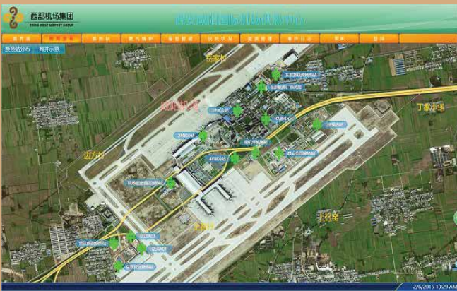
Heat Station Control Using EarthWorX™ GEO SCADA
