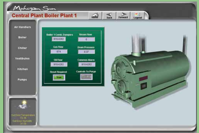
Boiler Plant Control
