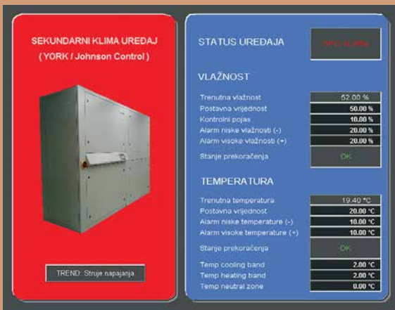
Air Conditioner Monitoring Screen in an Example Alarm Condition
