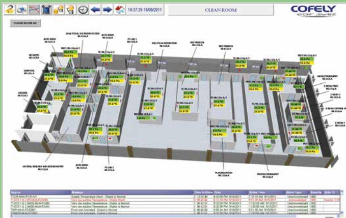
Clean Room Floor Monitoring/Control
