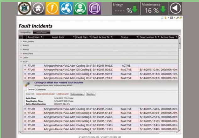
A Maintenance Alarm Screen Created Through ICONICS Facility AnalytiX
