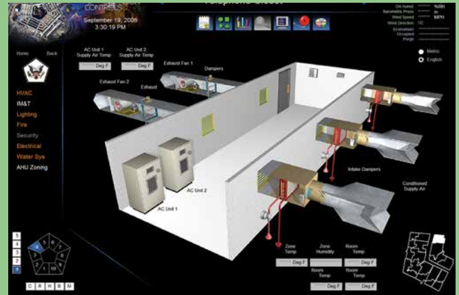
A Building Operations Control Screen
