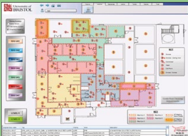
An AHU Zone Monitoring Display
