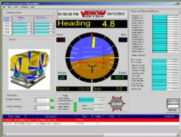
ROV Model Monitoring and Control by Hydrovision
