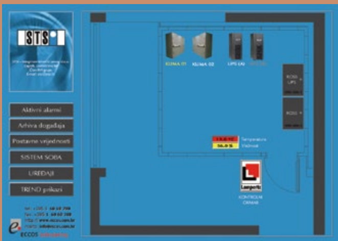
Main Screen for STSI d.o.o. Integrated Technical Services' Datacenter Control
