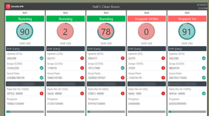
Figure 3: Departmental Overview of Shift OEE, Machine Status and Order Status Running on a Raspberry Pi
