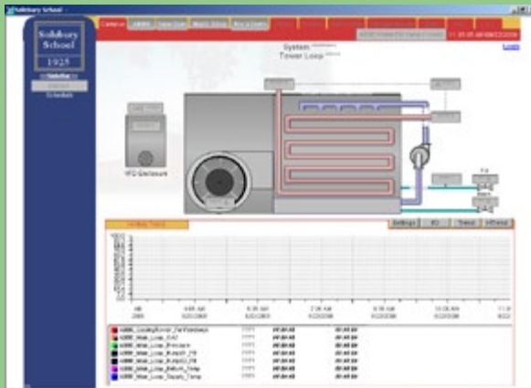
Cooling Tower Monitoring/Control Solebury School
